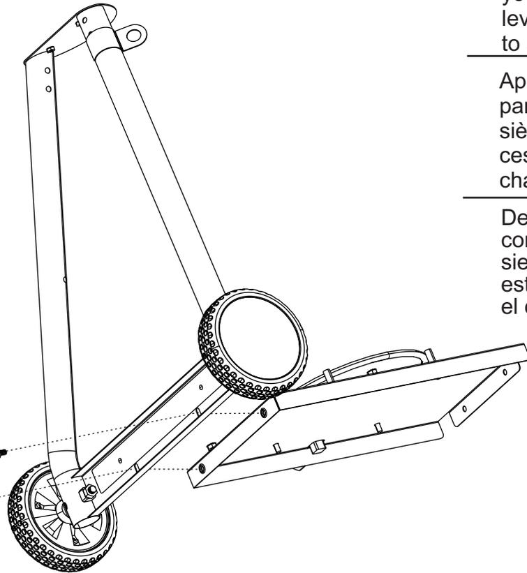
After cart assembly, if your cart does not sit level, use these screws to adjust the cart.
