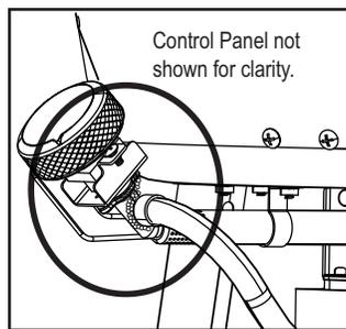
5. If "growing" bubbles appear, there is a leak. Close LP cylinder valve immediately and retighten connections. **If leaks cannot be stopped do not try to repair.** Call for replacement parts.
